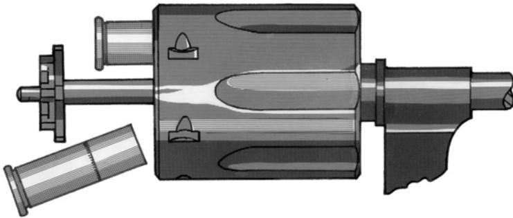
Trapping shell casings under the extractors of Smith & Wesson revolvers is caused by failure to hold the weapon with the muzzle pointed straight up when fully depressing and releasing the extractor rod. The frequency of occurrence seems to increase when reloading in stressful circumstances. Many law enforcement agencies have reported high incidences of this problem in stress training courses and in actual police shooting situations in the field.
