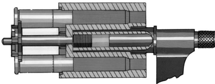
The modification can be made quickly and without any special tooling. It prevents the extractor from drawing the spent casings out of the cylinder far enough to allow them to fall under the extractor. When properly installed it will not affect any other function of the weapon.
