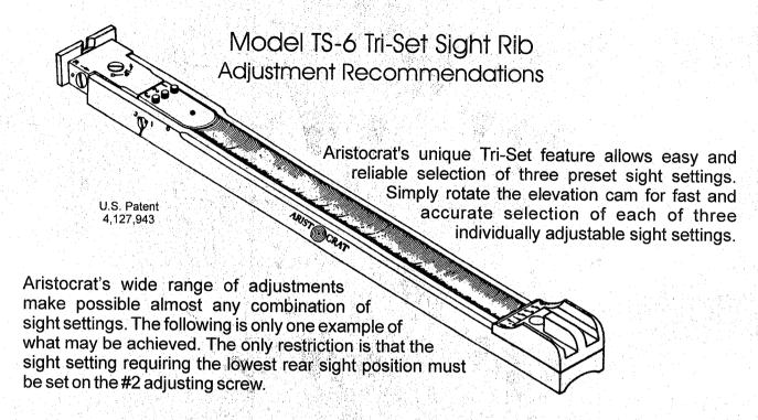
Sighting in is accomplished as follows: First turn the slotted elevation screw all the way to the bottom. Then rotate it back up approximately one half turn. This screw is not used again except to compensate for lighting or ammunition variables.
